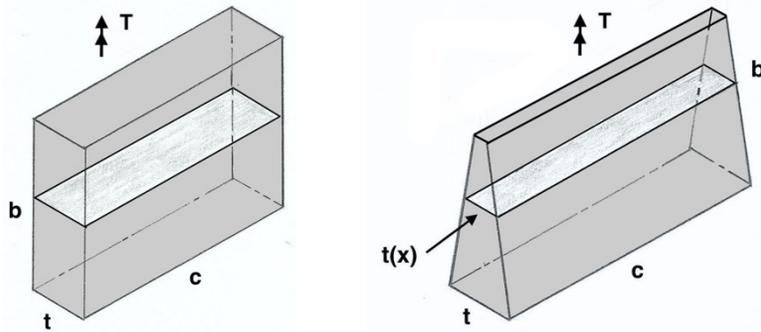
Figure-1, Flat fin geometry (left) compared to tapered fin geometry (right)
