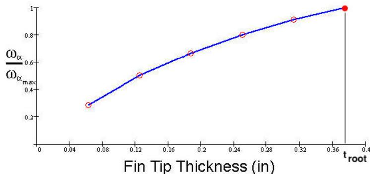
Figure-5, Ratio of tapered fin torsional frequency for fin-tip thickness that increases from 0.0625 inches at the tip to the root thickness specified as 0.375 inches
