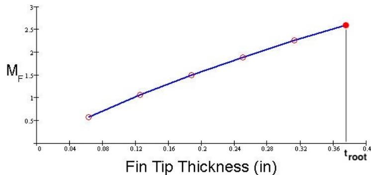
Figure-4, Flutter Mach number verses increasing fin tip thickness
