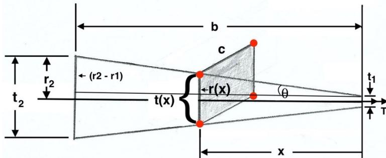
Figure-2, Tapered Fin:  $[x = 0, t = t_1]$ ,  $[x = b, t = t_2]$ ,  $\tan \theta = (r_2 - r_1)/b$
