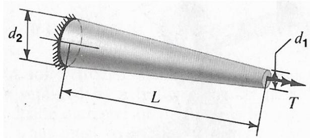
Figure-3, Solid, tapered shaft rigidly fixed at one end
